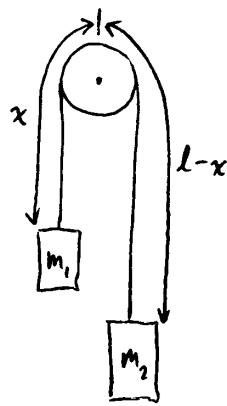
A frictionless pulley with two masses  $m_1$  &  $m_2$  hanging from it.
