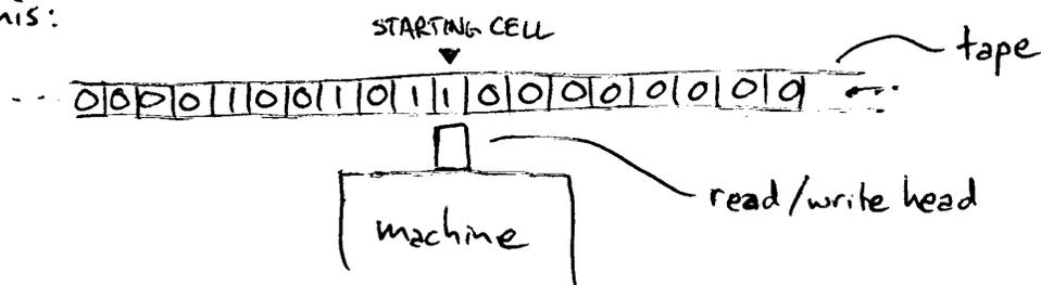
The machine has a finite set of states with distinguished start and halt states, & rules saying how at each step, the machine uses its current state & the bit on the cell the head is reading to:
