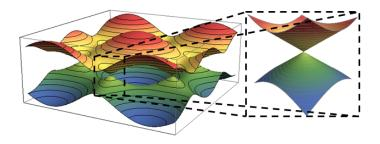
This shows the energy E of electrons moving in a sheet of graphene as a function of their momentum  $(p_x, p_y)$ . At certain points this looks like a lightcone in energy-momentum space. That's what we expect for a massless particle in special relativity!
