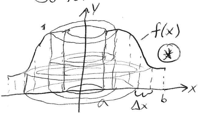
$$V_i = (2\pi \bar{x}_i) [f(\bar{x}_i)] \Delta x \\ V \approx \sum_{i=1}^n V_i = \sum_{i=1}^n 2\pi (\bar{x}_i) f(\bar{x}_i) \Delta x$$
