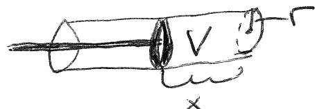
Solution:  $V = \pi r^2 x$  via picture.  $\Rightarrow V_1 = \pi r^2 x_1$
