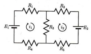
Write an equation that describes the sum of voltage drops around loop 1 (i.e., the loop with current  $i_1$ ).
