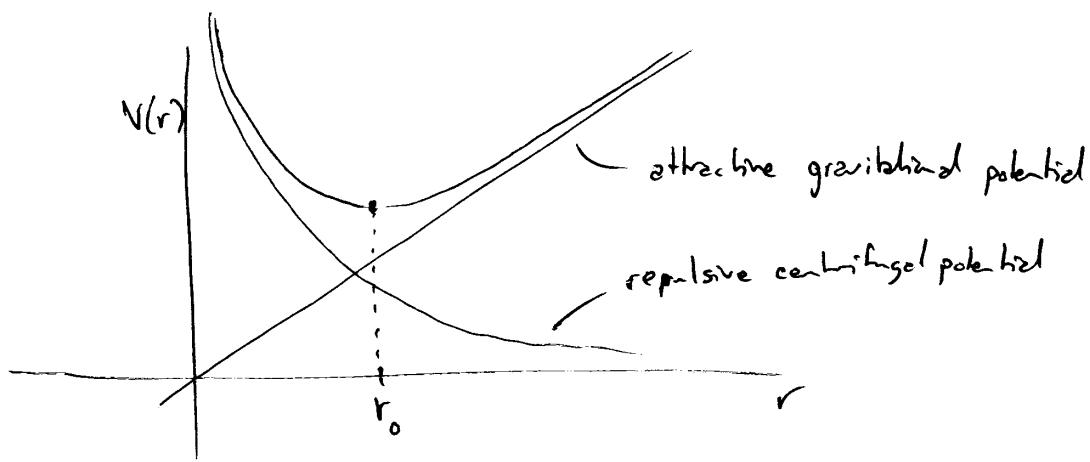
At  $r_0$ , the minimum of  $V$ , our mass  $m$ , will be in a stable circular orbit of radius  $r_0$  (which depends on  $J$ ). Otherwise we get orbits like:
