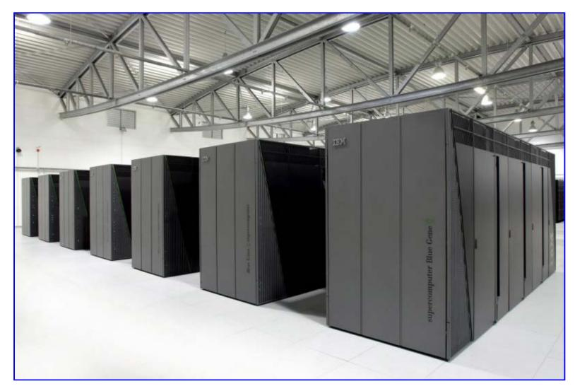
This computer is called <u>JUQUEEN</u>. You can see 7 big boxes here. Each box holds 4 racks. Each rack holds 16 boards. Each board holds 32 nodes. Each node has 32 cores.
