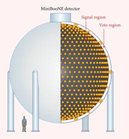
MiniBooNE: 800 tons of mineral oil in a tank bombarded with muon neutrinos from a distance of 500 meters... for 16 years.
