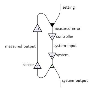
Feedback is the most important concept in control theory: letting the output of a system affect its input. For this we should let wires 'bend back':
