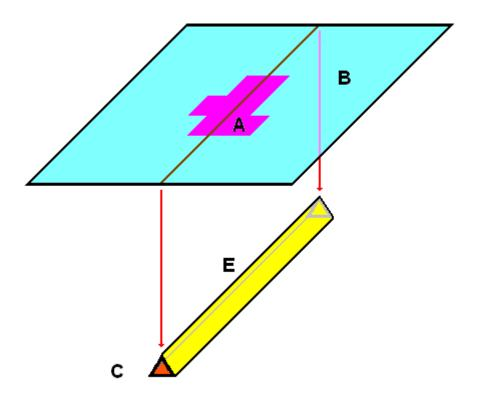
Since we are resting **A** and **B** along a line containing the center of mass for this combined physical system of objects, *we expect that the combined object will balance perfectly*, not tipping either to the left or right.
