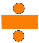
One can start the construction by attaching the top and bottom disks to the rectangle at single points of tangency.
