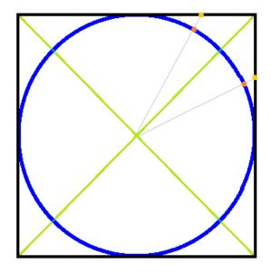
In the drawing, a point on the circle is a dark orange dot and its image is a light orange dot. An inverse mapping is apparent from the picture; we merely reverse the preceding construction, starting with a point on the boundary of the square and taking the point on the line segment joining that point and the center at which the segment meets the circle. To show that we really obtain a homeomorphism in this manner, as usual it is necessary to translate the picture into algebraic formulas.
