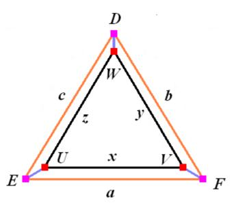
If we apply the formulas for resistances in series and parallel, we obtain the following system of three equations in x, y, z in terms of a, b, and c.
