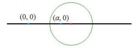
The two points are indicated by blue dots, the locus is the circle in the drawing, and the center of the circle is indicated by the red dot. As noted above, the center of the circle has coordinates (4a/3,0) and the radius of the circle is equal to 2a/3. This circle meets the x – axis at the points (2a/3,0) and (2a,0).
