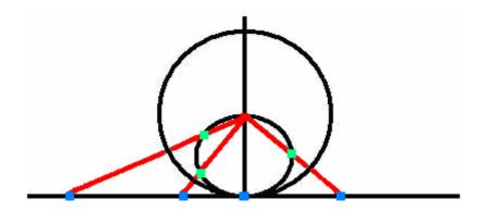
This drawing illustrates an arbitrary 2 – dimensional cross – section of a stereographic projection, with the set of all points on the small circle (except for the point at the top) being mapped to the common tangent line for the two circles in the picture. The designated points, where the rays meet the small circle and the tangent line, correspond under stereographic projection and its inverse, and they also correspond to each other under inversion with respect to the larger circle.
